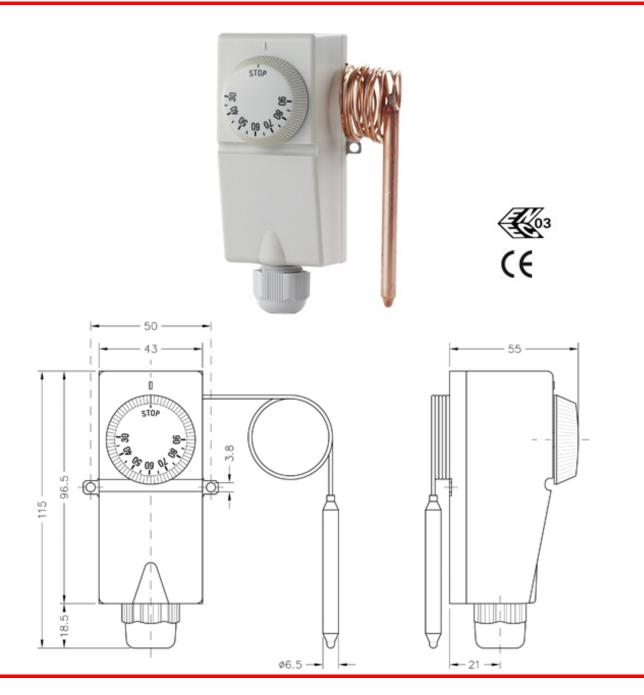
**TUREC** is a boxed unipolar thermostat, liquid expansion, with switching contacts, complete with core hitch. Ideal for automatic regulation on boilers, pumps and other heating equipment. The thermostat can be fixed on any surface using the perforated fins. The temperature sensor is the bulb at the end of the capillary which you must immerse in the liquid (or place it closely touching the surface) that the temperature has to be regulated for.
